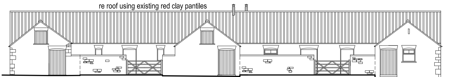
south elevation natural coursed stonework and joints to match existing natural coursed stonework and joints to match existing
